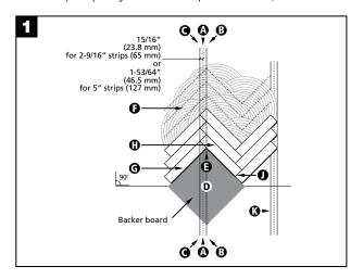
Notes: Only cover surfaces that can be reasonably laid in two hours (maximum 5 rows), since adhesive may dry too quickly and not stick properly. Reaction time may vary from one adhesive to another and may also be affected by room temperature and relative humidity (see manufacturer's specs on container).
